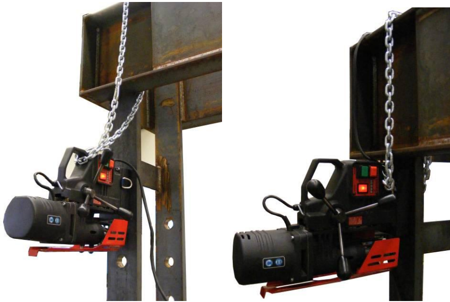
Drawing 1. Examples how safety chain should be fastened..
