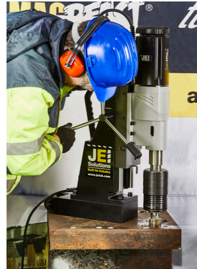
MagBeast 5 in action with tapping chuck and clutched collet
