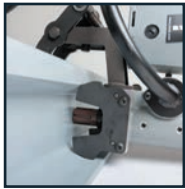
Featuring clamp and Turbo rail cutter
