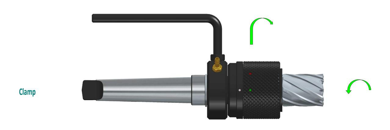
Step 3: Rotate the clamping sleeve anticlockwise as shown by the arrow. Turn the "red mark" to the same horizontal line as the "white mark" to remove annular cutter.
