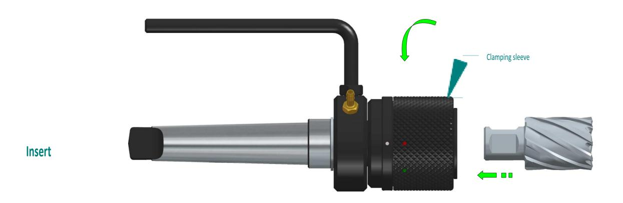
Step 2: Install one flat of cutter shank into arbor by corresponding the "white mark", loosen the clamping sleeve. The "green mark" correspond to the "white mark", which is automatically fixed.
