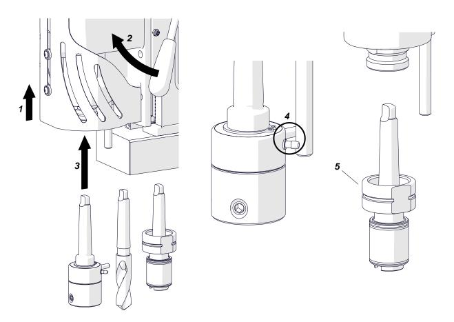
To remove the arbor (drill bit, tap chuck), continue as follows. If the arbor (tap chuck) has a nut (1), remove the nut. Next, lift the motor and rotate the spindle (2) to align the holes in the spindle and gearbox (3). Put the drift into the hole (4). Next, hold the carrying handle with one hand and hit the drift with a mallet (5).
