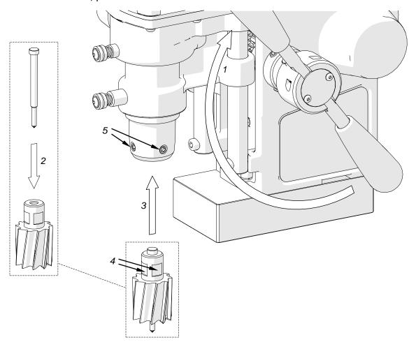
**Figure 3.** Mounting the annular cutter
