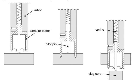
Figure 4. Annular cutters operation
