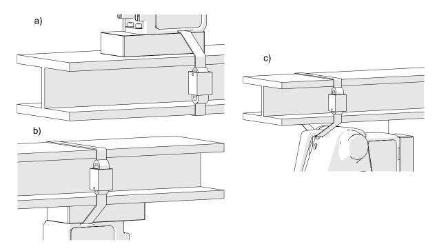
**Figure 7.** Securing the drilling machine using the safety strap
