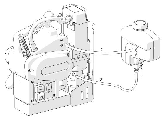
Figure 6. Mounting the cooling system bottle
