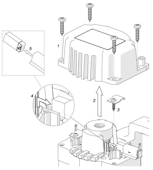
Figure 9. Replacing the brushes
