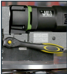
Ratchet handle for left or right sided operation
