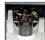
Milling inserts 4 sided for long tool life
