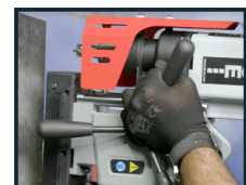
Self-correcting slide rails
