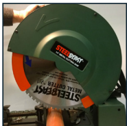
Retracting lower safety guard
