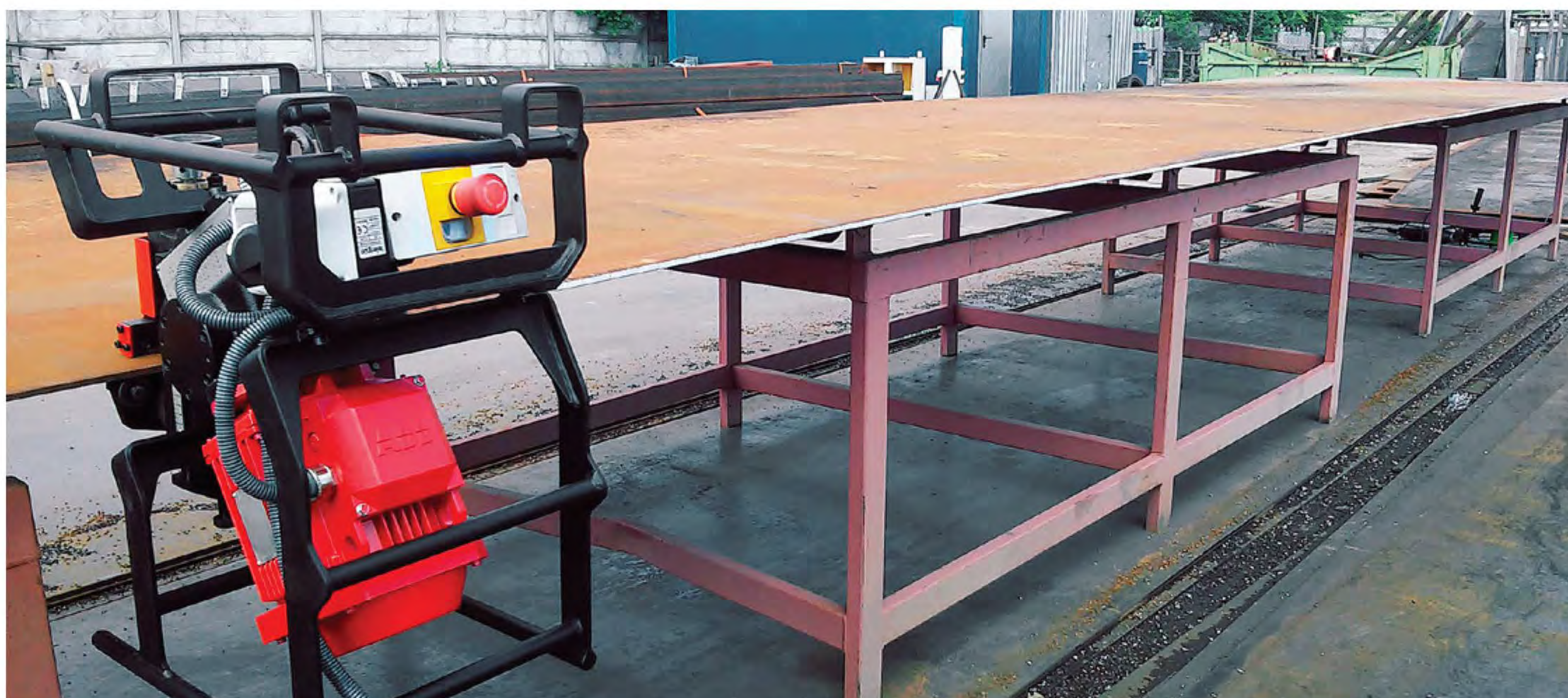
ABM-14 runs along a plate automatically
