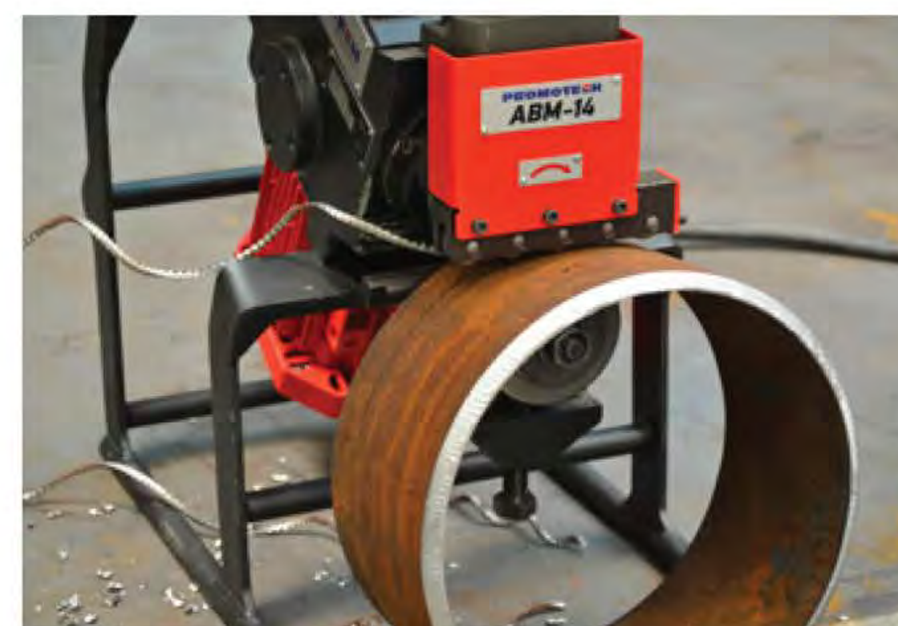
Oval workpiece and pipe beveling
