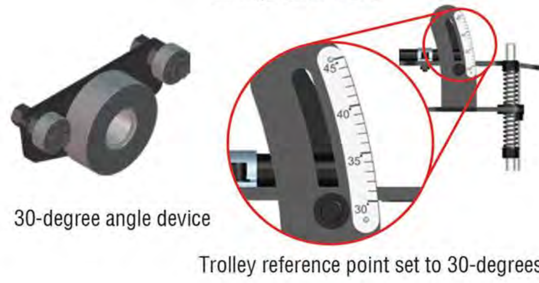
Top beveling at 30 degrees Configuration 1 or 2
