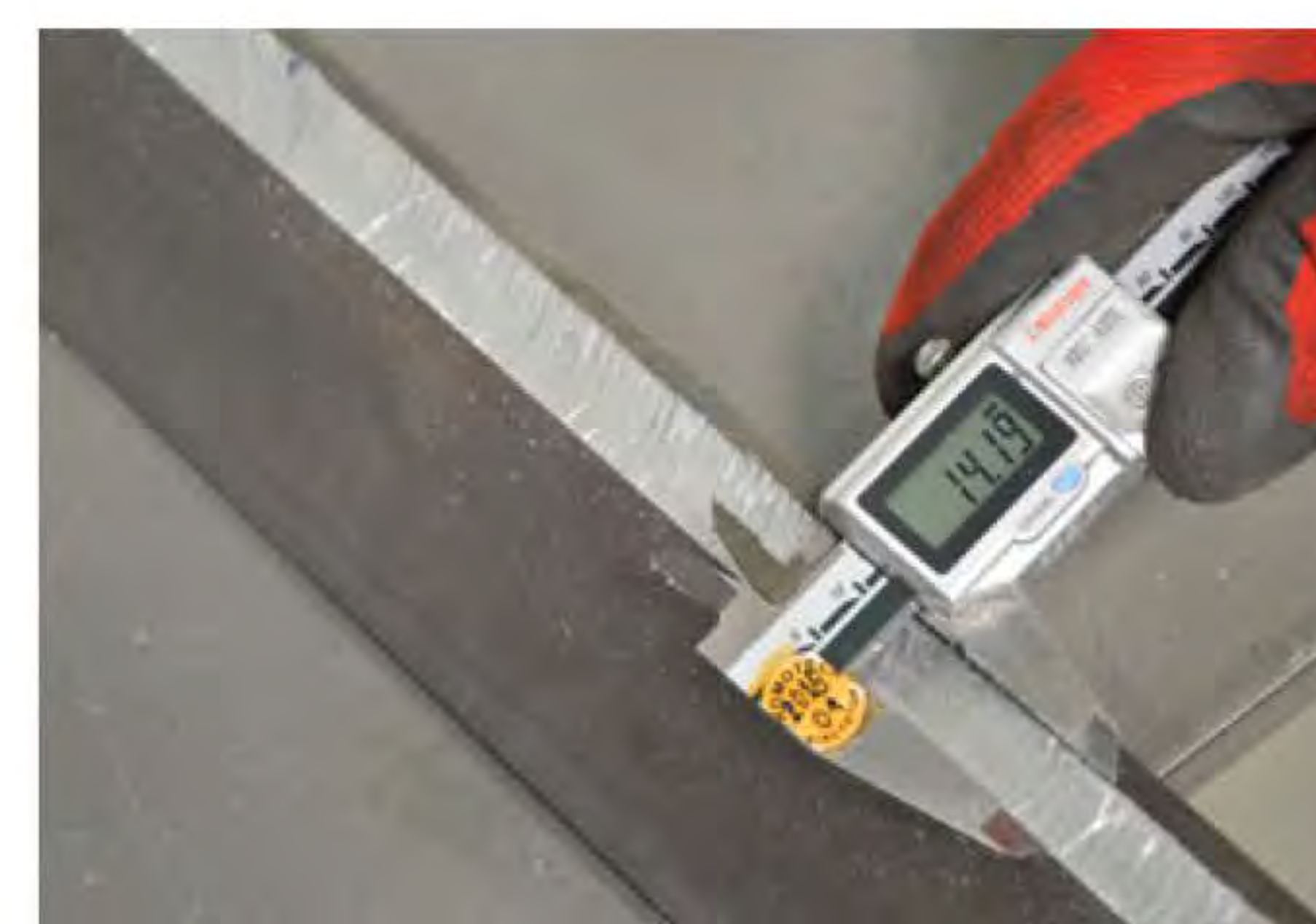
Maximum bevel width up to 14 mm
