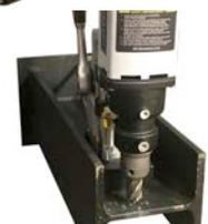
Ability to position machine to drill in tight access corners.
